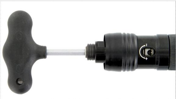
Slide cover to the front. Use wrench to rotate the shaft until you can see the hole for the wrench.
