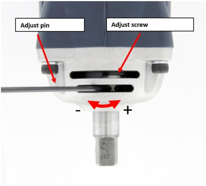
The adjust screw is blocked in both directions, never use force or otherwise the screw or internal parts may get damaged.
