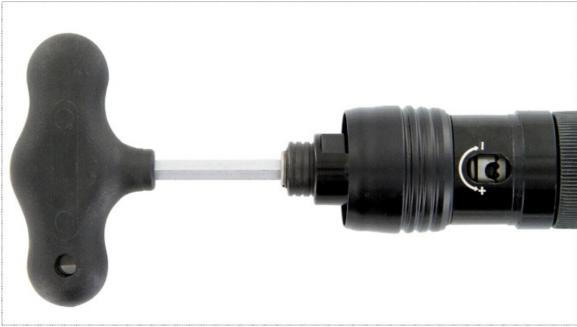
Slide cover to the front. Use wrench to rotate the shaft until you can see the hole for the wrench.
