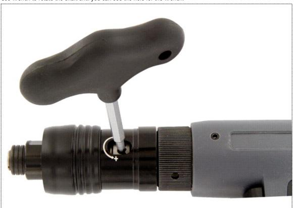
Insert the wrench in the hole. Rotate the wrench counter clockwise to increase the torque (+).
