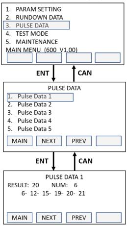
Result: 20 = the average on which the tool has shut-off.
