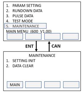
Selecting SETTING INIT or DATA CLEAR with the up and down arrow and press ENT.
