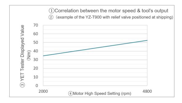
The above shows the influence of the motor speed on the torque output, this is an example of the YZ-T900 tested on the static torque tester YET-1001C.
