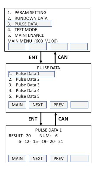
Result: 20 = the average on which the tool has shut-off.
