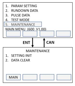
Selecting SETTING INIT or DATA CLEAR with the up and down arrow and press ENT.
