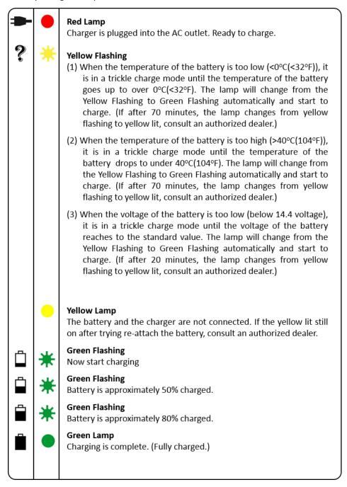
Please remove the battery from the tool at the end of the working day or before the weekend. The battery may be de-charge during longer period of times when mounted on the tool. This may cause a too deep de-charged battery and this may trouble re-charging the battery: See pont nr. (3) above.
