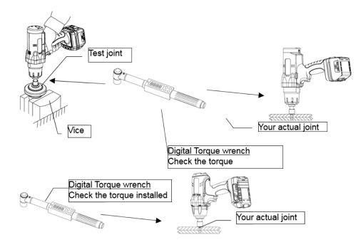
Test method 2: dynamic measurement with a rotary torque transducer on a test joint.
