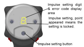
Push the button for 2 seconds until the number starts blinking.
