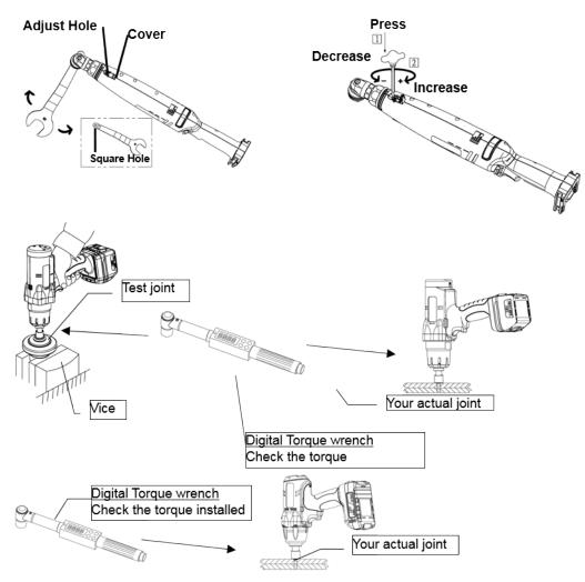
Test method 2: dynamic measurement with a rotary torque transducer on a test joint.
