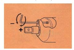
The oil in the impulse unit must be regularly replaced. Preventive maintenance is important because if the oil is replaced too late the viscosity changes so the torque will decrease and damage may occur on the internal parts.
