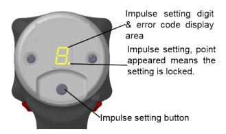
Push the button for 2 seconds until the number starts blinking.
