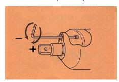
The oil in the impulse unit must be regularly replaced. Preventive maintenance is important because if the oil is replaced too late the viscosity changes so the torque will decrease and damage may occur on the internal parts.
