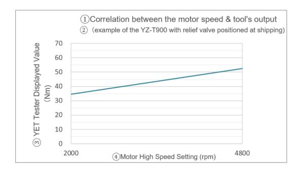
The above shows the influence of the motor speed on the torque output, this is an example of the YZ-T900 tested on the static torque tester YET-1001C.
