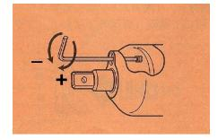
The oil in the impulse unit must be regularly replaced. Preventive maintenance is important because if the oil is replaced too late the viscosity changes so the torque will decrease and damage may occur on the internal parts.
