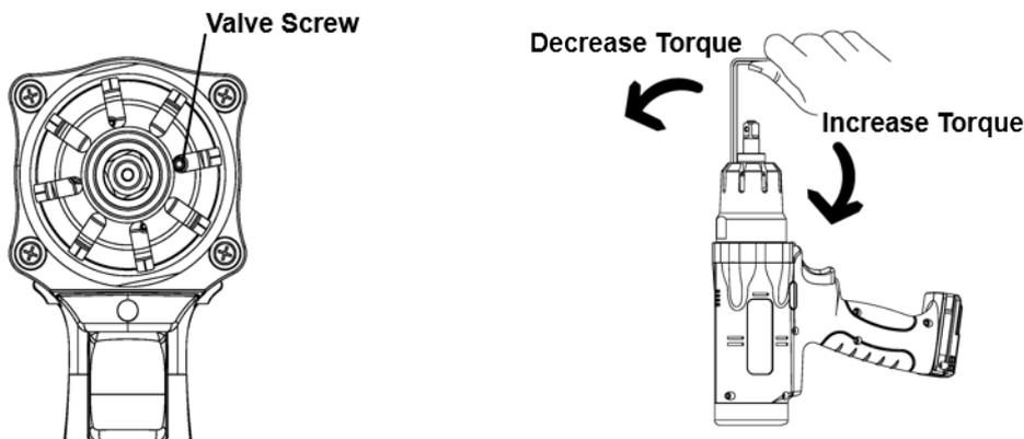
**How to test the torque**
