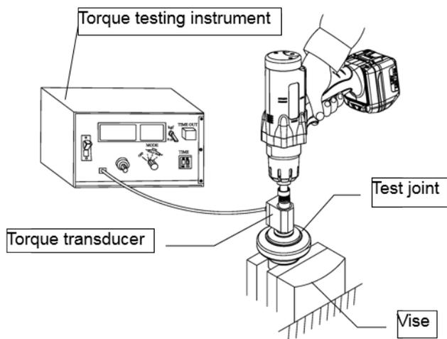
Test method 3: dynamic measurement with a rotary torque transducer on the actual application.
