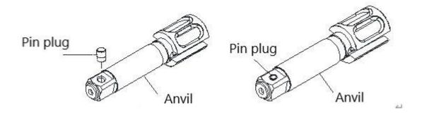
2. After pushing the pin plug inside, turn the anvil to the other side, and push in the spring(I100-506), pin(33255-WRBA-01) and washer(33239-WRBA-08) one by one. The pin retainer set is now completed.
